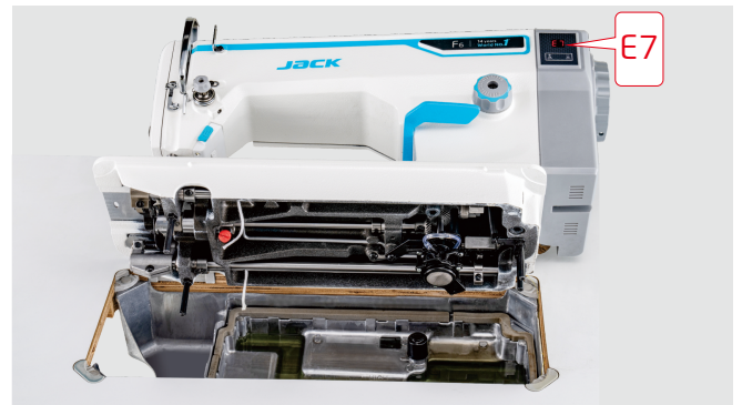
Safety Switch : After turning on the machine, an error is displayed to prevent accidental operation from injuring people
